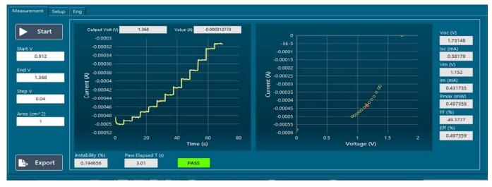
NREL Asymptotic measurement for perovskite solar cells. IVS-KA6000 has a unique "asymptotic method" test function. The "asymptotic method" has become one of the standard methods for efficiency testing of new solar cells. IVS-KA6000 has a complete "asymptotic method" supporting scheme and automatic program control.
